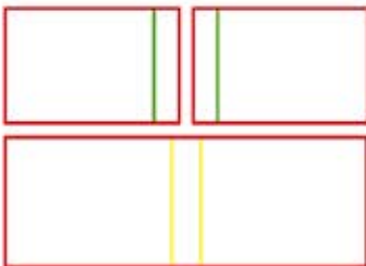
The images are perfectly aligned when the green and red guidelines (right) overlap and turn yellow (below)
